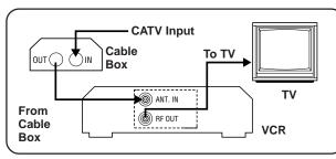
With this connection you can view/record any cable channel <u>including scrambled channels to</u> which you have subscribed.
