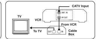
With this connection, you can view one scrambled cable channel while recording another unscrambled channel.
